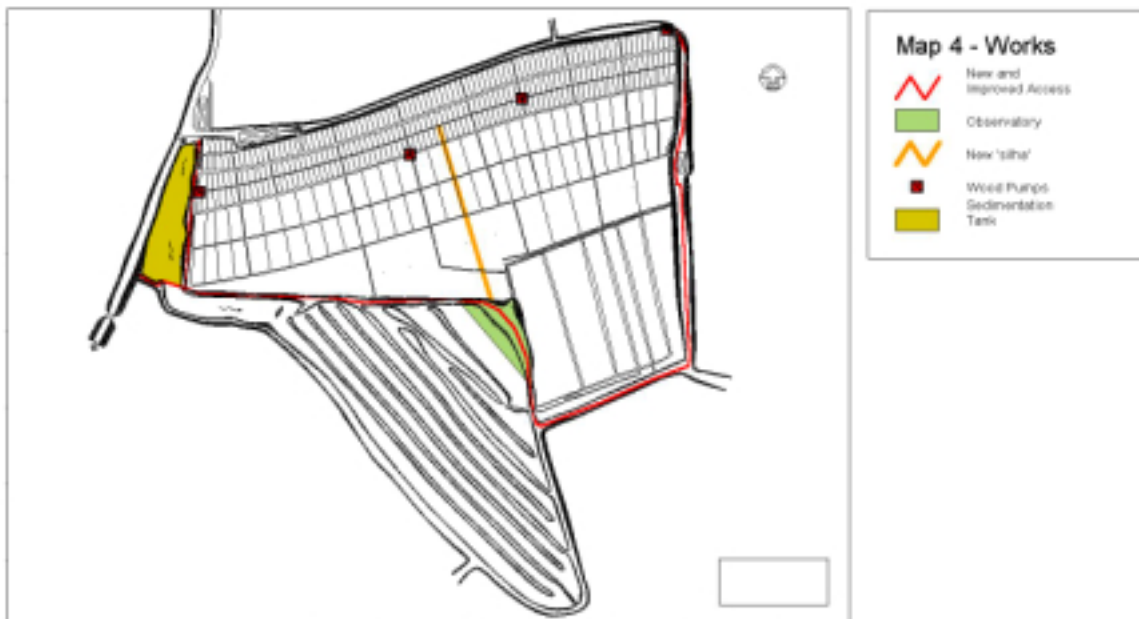
Figure 14 - Works I - Cleaning and improving access ways (red line); sediment deposited for observatory (green); construction of new silha (yellow line); reconstruction of pumps (red squares); sedimentation tank (yellow area)
