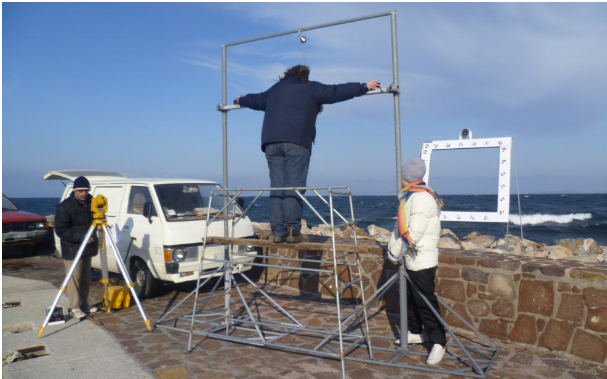
Figure 2. The general system configuration with the target frame, the camera platform and the total station.
