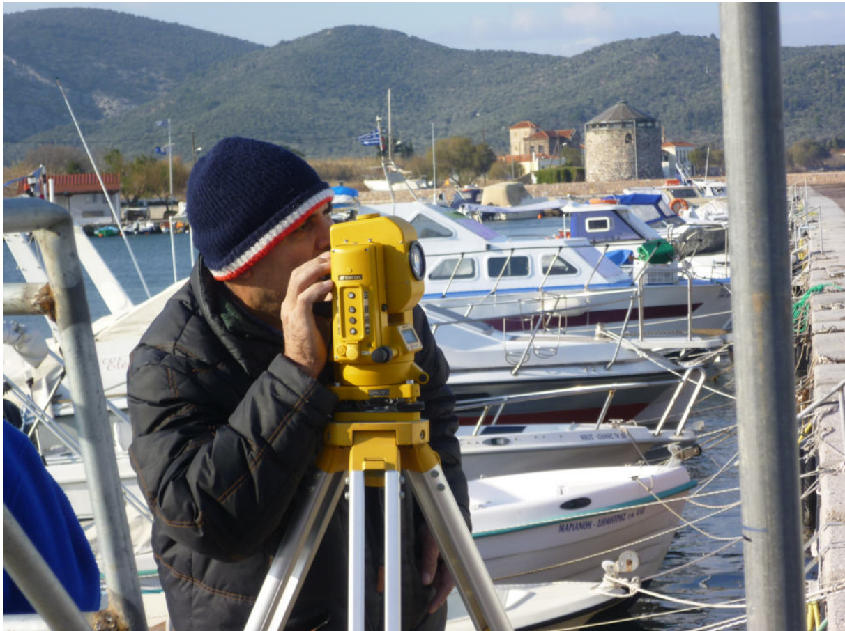
Figure 3. Total station surveys to establish control on the target frame.
